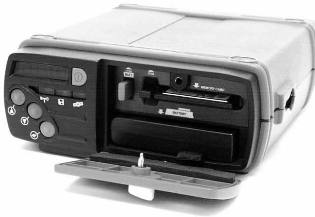
Figure 3.2. Installing an Internal Battery
