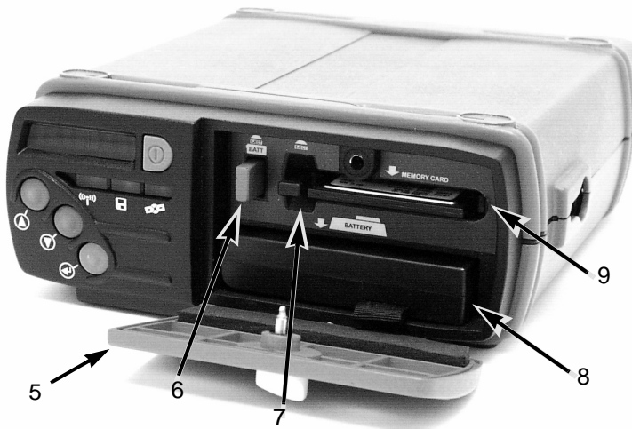
Figure 2.2. Z-Xtreme Front Panel Open
