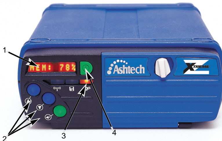
Figure 2.1. Z-Xtreme Front Panel Closed
