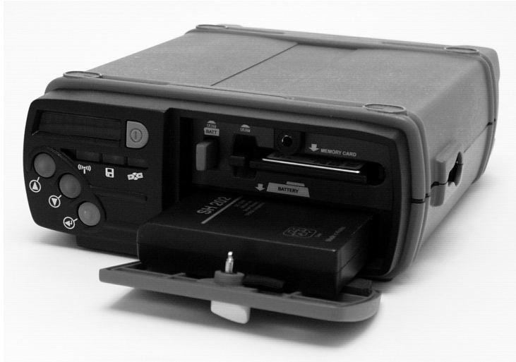
Figure 3.3. Removing an Internal Battery
